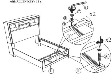
STEP 6.1: Insert the Drawer (J) at the Drawer Support Rail (I). STEP 6.2: Remove HANDLE and using a Philips head screw driver as shown
